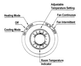
Activating the "SYSTEM OFF" switch should be done with care because there will be no heating or cooling operation even though there may be a demand - a room could potentially go into a freezing condition. Once a comfortable temperature setting is established, no other adjustments are necessary, except for fan speed, which is adjusted using the fan speed control knob at the unit.
