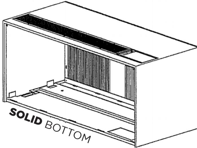
EA, RS and ES chassis can be installed into original SOLID BOTTOM sleeves, if the correct front covers are used.
