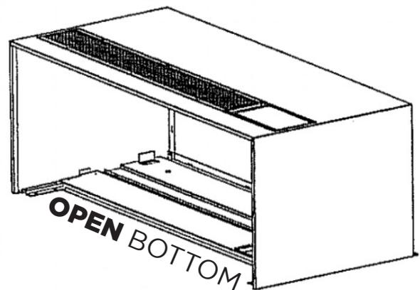
When installing EA, RS, and ES replacements, ensuring proper evaporator airflow is critical. The following 2 pages describe the front panels and retrofit kits that are available to ensure proper installation depending on the combination of sleeve type (Solid or Open Bottom) and desired chassis type (EA Electric, RS Heatpump, ES Electric).
