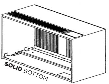
EA, RS and ES chassis can be installed into original SOLID BOTTOM sleeves, if the correct front covers are used.
