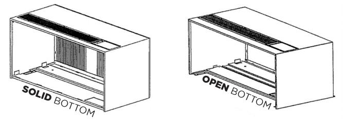
When installing EA, RS, and ES replacements, ensuring proper evaporator airflow is critical. The following 2 pages describe the front panels and retrofit kits that are available to ensure proper installation depending on the combination of sleeve type (Solid or Open Bottom) and desired chassis type (EA Electric, RS Heatpump, ES Electric).
